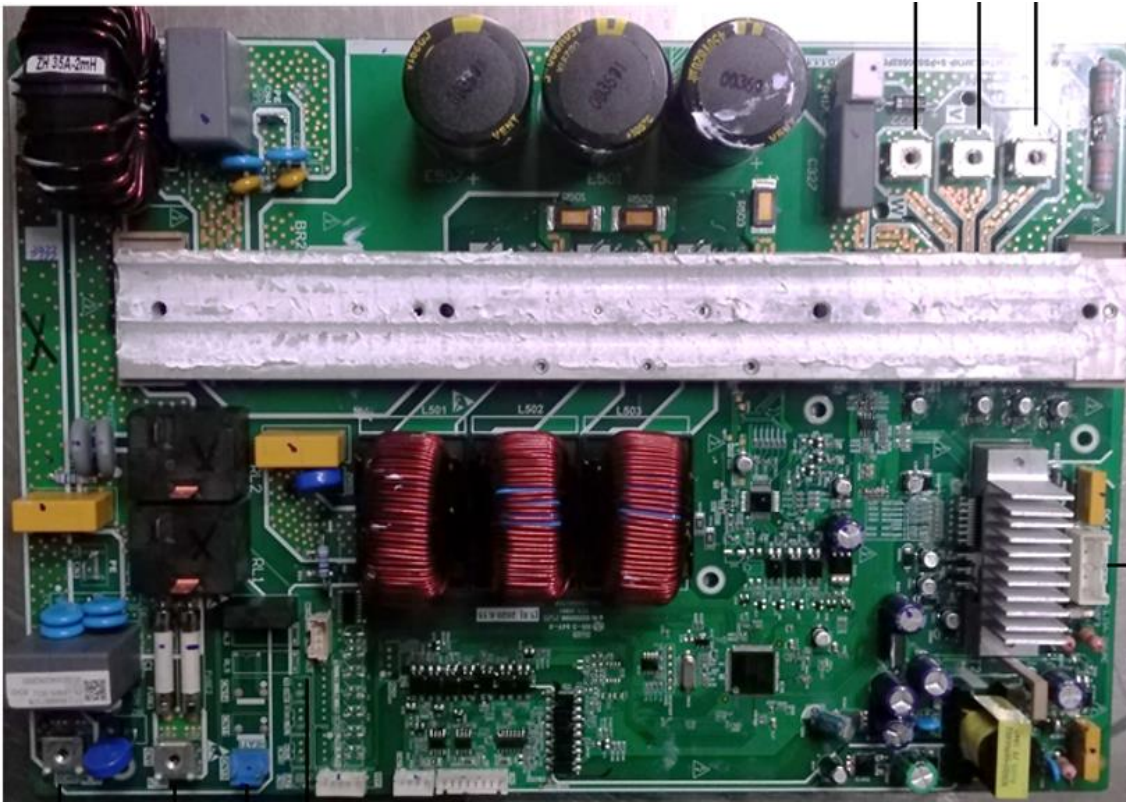
Figure 4-1.4: 36/42/48/56 model outdoor unit communication switchboard
